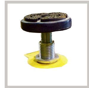
Rubber covered drop in style double adjusting lift pads
