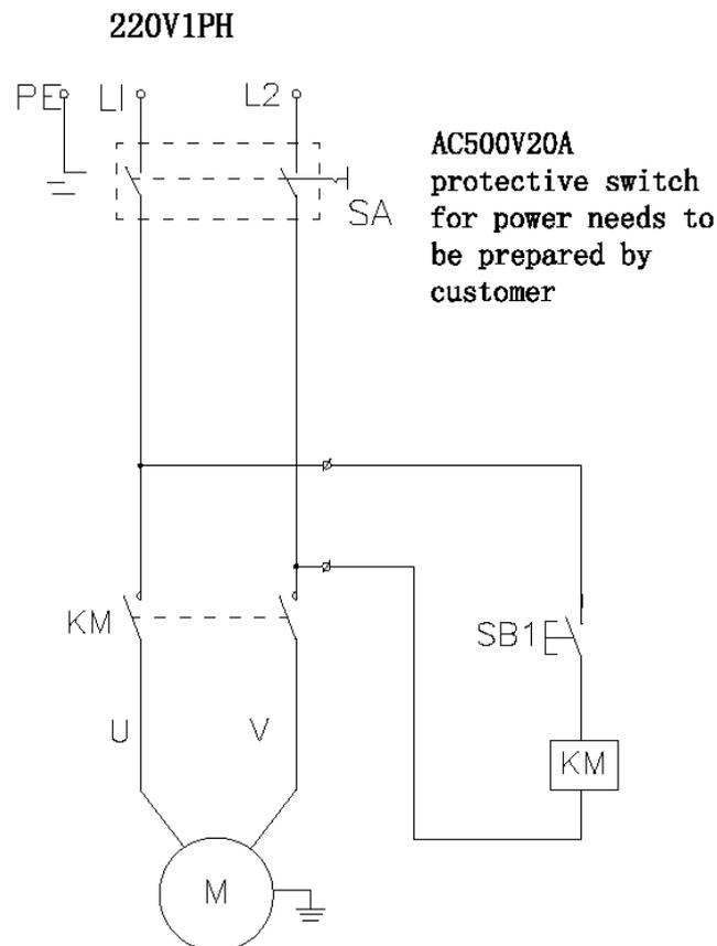
M-Motor    KM-Contactor    SB1-Button
