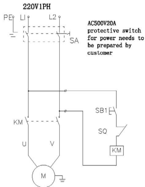
M-Motor KM-Contactor SB1 –Button SQ- Limit switch
